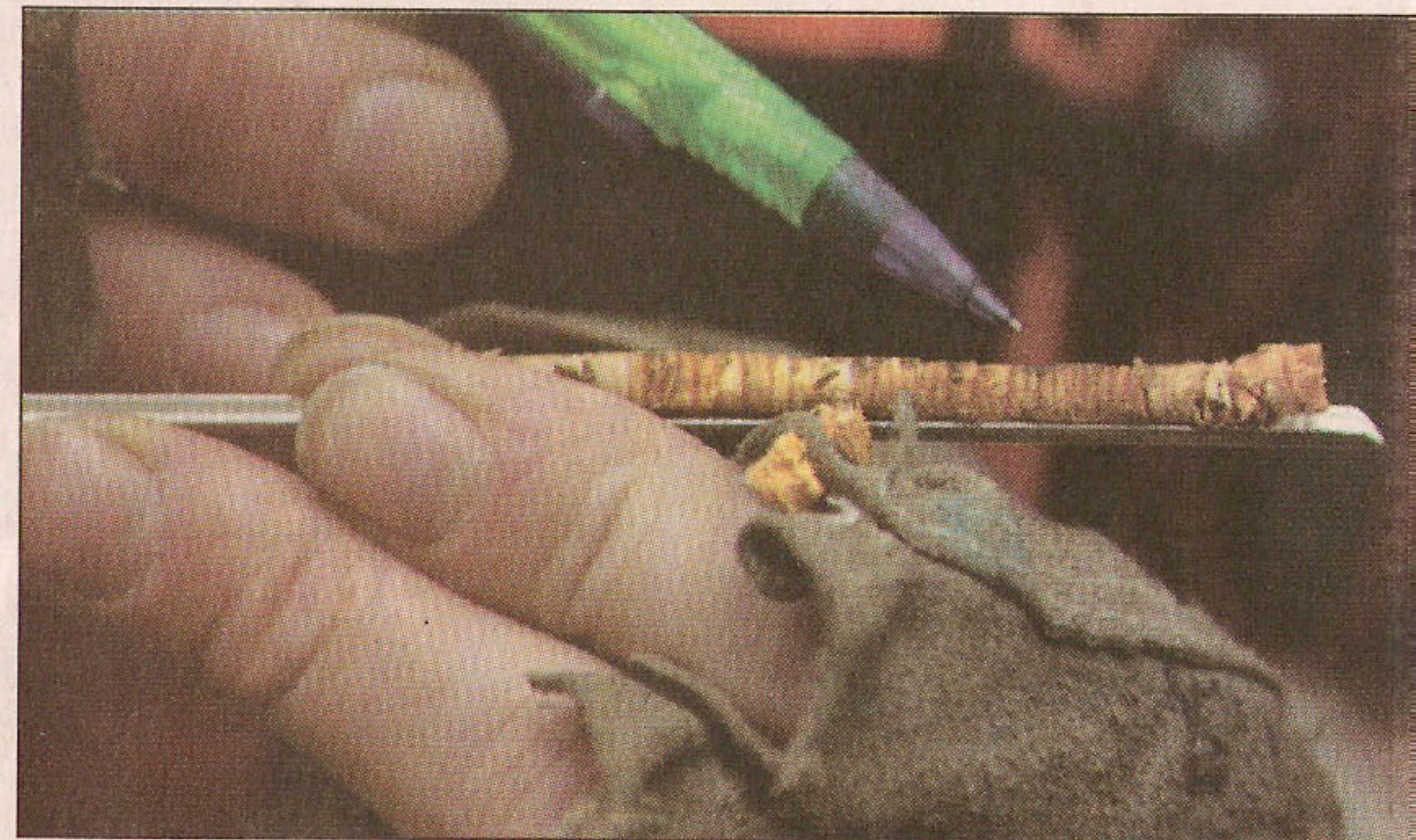
A tool called an increment borer extracts a core sample from a young cedar on Long Island. The rings reveal the tree is 54 years old.
